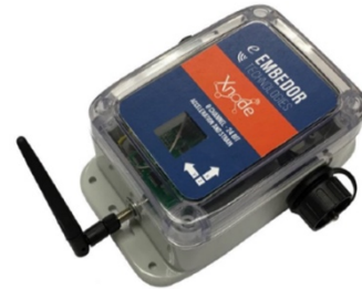
Figure 2 - StructureIQ's SHM Wireless sensor
